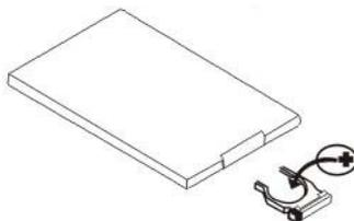
2. Put the button-type battery (+) mark upward into the battery holder.
