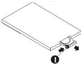
1. Pull out the Battery Holder while pressing the stopper.
