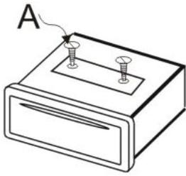
Note: Remove the protection screws (A) before installing and operation the unit.
