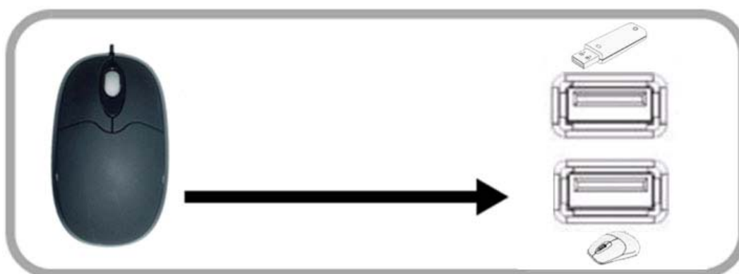
Connect a USB mouse to the bottom USB port on the front panel
